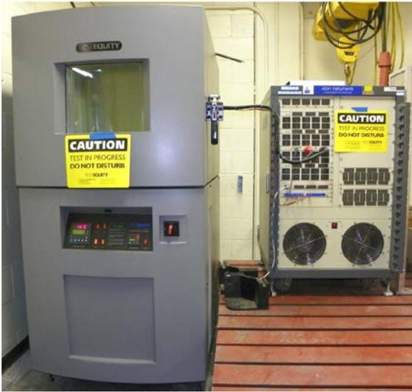
FIGURE 6. BATTERY CYCLER AND TEMPERATURE CHAMBER
